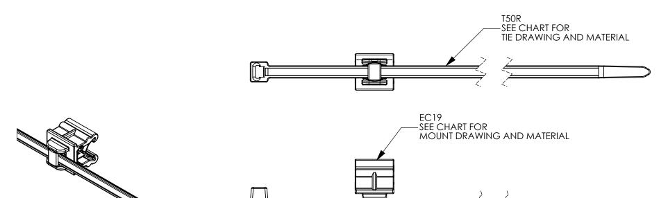
DELIVERY CONDITION: CABLE TIE HEAD COULD BE AT THE LEFT OR RIGHT SIDE OF EDGE CLIP
